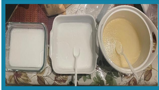
**Figure 1.6 - Experimental Setup. The three containers each contain one MF filter sponge soaking in the polymer.**
